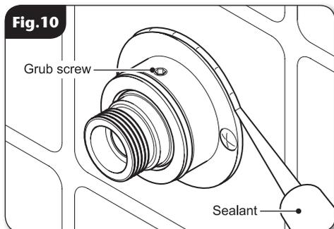
Align the mounting plate fixing holes to the intended position and mark the holes.
